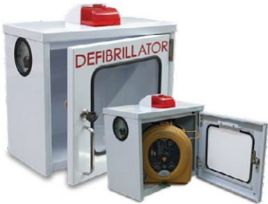
AED Cabinet Model : PM-01-AC Size : 330mm(L) x 160mm(W) x 300mm(H) Weight : 3.9 kg Product Description : • Included with Siren Sound and Light • Allow to mounted on wall • Break glass to get the key • Include with 9V battery and 2 keys *AED not included
